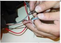
Second possibility is: One blue(+) and one black(-) that will power up both halos and leds or just the halos if leds are not present.
