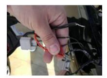
Step 3: Splice the red wire (+) from the head light to the (+)positive wire of the stock harness.
