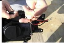
One possibility is two sets of wires A. One red wire (+) and one black(-) for the halos. B. One red wire(+) and one black(-) for the leds.
