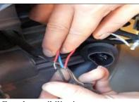
Fourth possibility is: A. Two red wires for the halos one red wire (+) and other red wire (-) or vise versa polarity does not matter. B. One red wire (+) and one black (-) wire for the leds.
