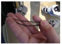
Pictured above is a parking light bulb harness. Depending on the vehicle you will have a different color wires for the power(+) and negative(-).
