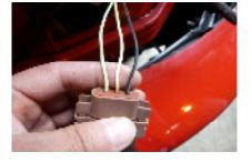
Step 2: locate the side maker or corner parking light pull back the electric tape to expose the wires on the stock harness. Your wire color configuration will vary from vehicle to vehicle.
