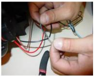
Step 4: Splice the black (-) wire from the head light to the black (-) wire to the stock harness.
