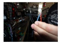
Step 1: Twist the two red wires together and the two black wire together from the Anzo headlight assembly. This step will vary depending on the which wire setup comes with the headlight assembly.
