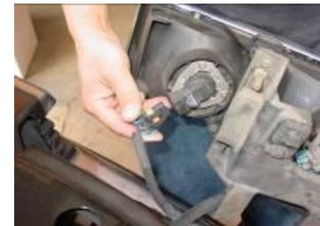
Step 6: Take the anzo headlight, splice in the red wire to blue and red wire to black to power up the halo's
