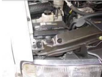
Step 1: Locate the two clips located at the top of the headlight.
