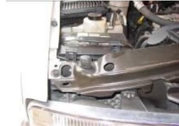
Step 2: Remove the two clips which hold the headlight to the frame.
