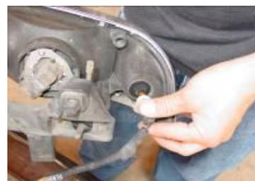
Step 5: Remove the parking light socket from the headlight.
