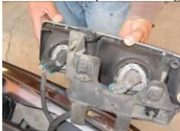
Step 4: Unplug the high and low beam harness from the bulbs.
