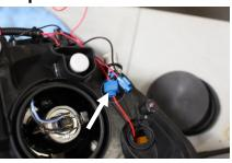
Connect the two wires from step 9 to the red wire from the parking light by using the wire splice connector
