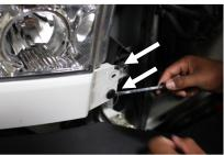
Locate the two trim pins on the lower headlight trim panel and remove the two pins
