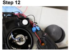
Connect the two wires from step 10 to the black wire from the parking light by using the wire splice connector
