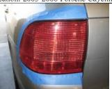
Step 1: remove the two plastic screw covers with the flat head.
