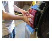
Step 6: Put new light in place and screw in the hex screws.
