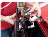
Step 3: Twist off the light bulb socket from the third brake light.
