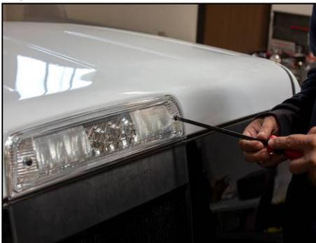
Insert Anzo USA 3<sup>rd</sup> brake light onto vehicle and screw factory screws into vehicle.
