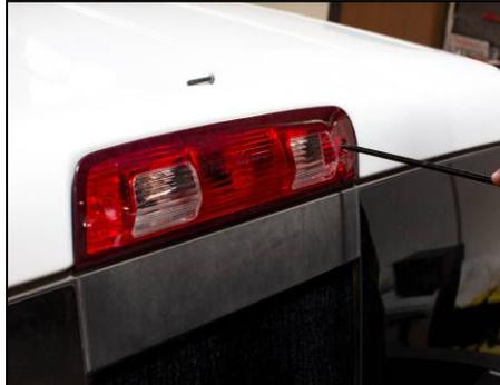
Use Phillip's head screwdriver to remove 2 screws holding factory 3<sup>rd</sup> brake light in place.
