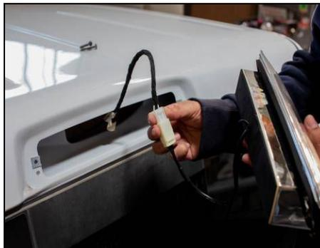
Connect main harness connector from vehicle side to Anzo USA 3<sup>rd</sup> brake light connector.
