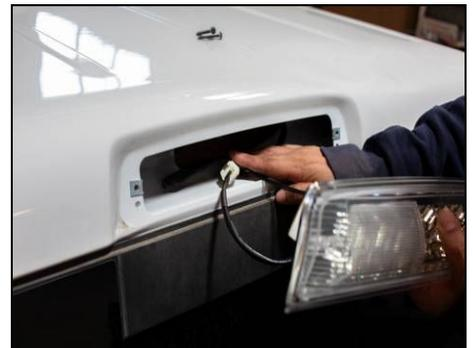
Insert resistor and main harness connector into opening.
