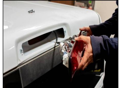
Remove factory 3<sup>rd</sup> brake light from vehicle.
