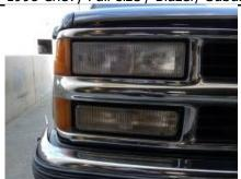
Step 1: Remove the four phillips screw holding in the parking light.
