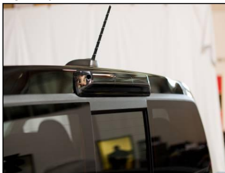
Slide Anzo USA 3 rd brake light into opening then tighten T15 torx screws by hand. *Do not over tighten*
