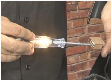
To check the polarity of the wires, you can use a light testing tool to check. First turn on the turn signal and ground your light testing tool and insert the tip of the tool into the socket. When the light testing tool flashes you have located the (+) positive turn signal wire.
