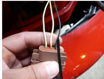
Locate the black (-) negative wire from the AnzoUSA headlight and splice that wire into the (-) negative wire on the turn signal harness, typically this wire will be black.
